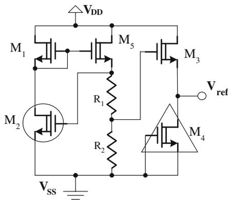
**Fig. 22** CMOS voltage reference based on N-channel MOSFETs gate work function difference proposed by Watanabe et al. [15]. Circle indicates  $p^+$  gate, triangle indicates  $n^-$  gate, all others are  $n^+$  gate
