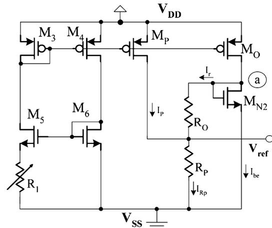
**Fig. 18** CMOS voltage reference circuit proposed by Pleterssek [26]
