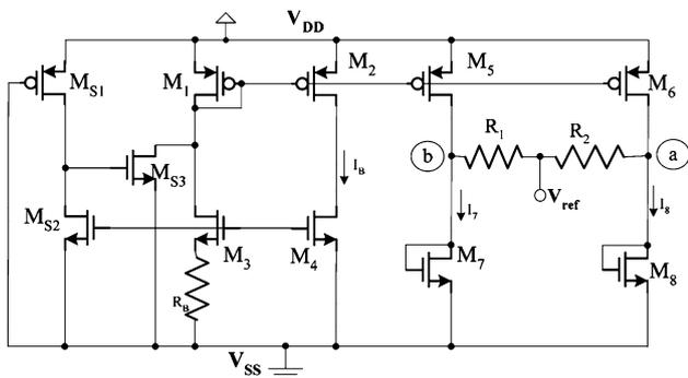
**Fig. 15** CMOS-based voltage reference using the zero temperature coefficient point proposed by Najafizadeh et al. [24]
