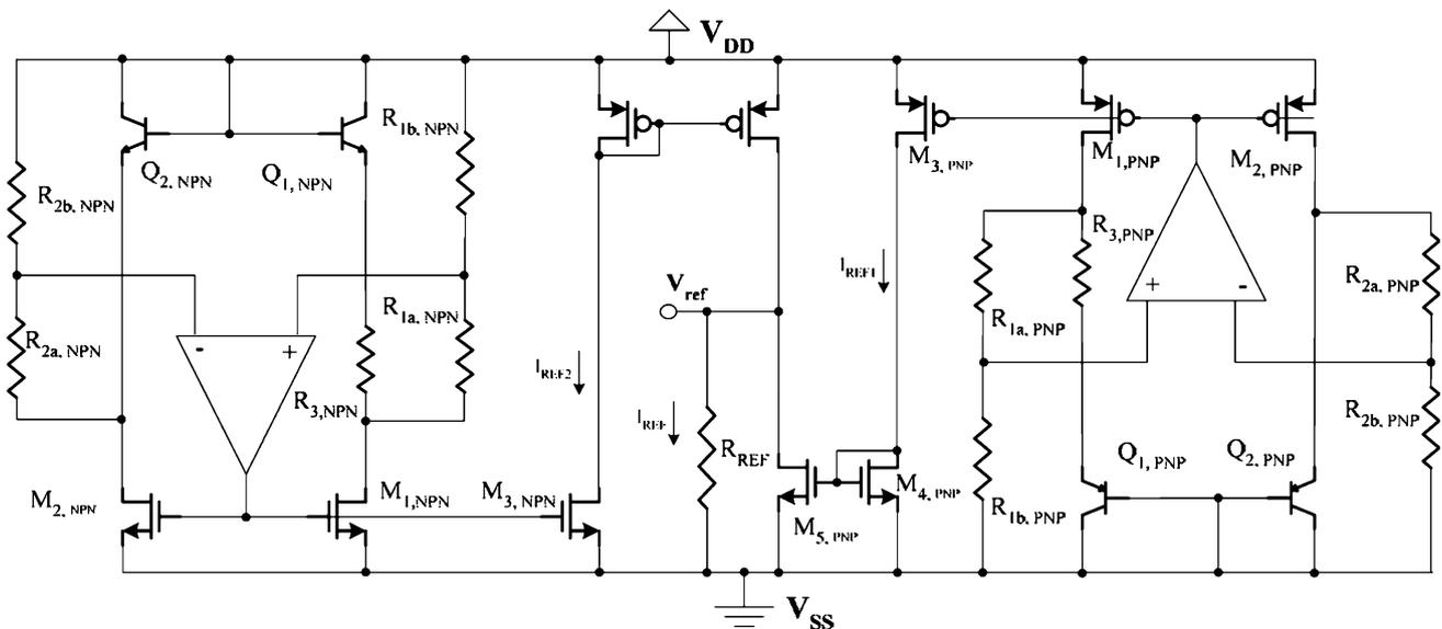
**Fig. 11** Curvature compensated a bandgap voltage reference proposed by Ker et al. [20]
