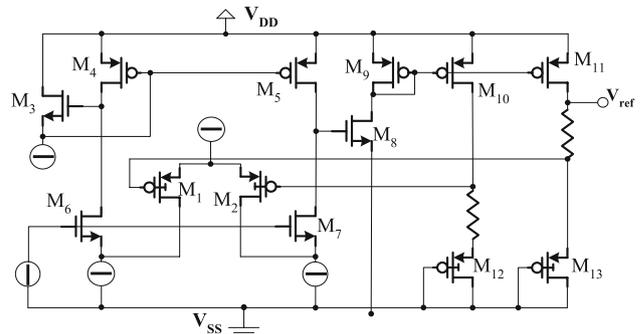
**Fig. 23** DTMOS-based voltage reference based proposed by Annema [16]
