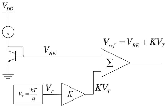
**Fig. 1** Block diagram of a bandgap voltage reference
