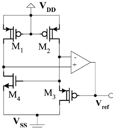
**Fig. 19** CMOS/SOI voltage reference circuit proposed by Ugajin et al. [14]
