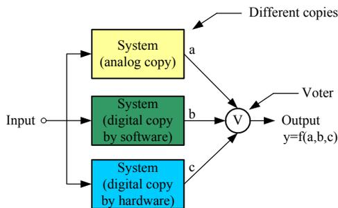
Figure 1. Mixed-Signal DTMR architecture.
