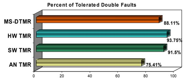
Figure 2. Comparison between the tolerance levels of the MS-DTMR scheme and traditional TMR systems.
