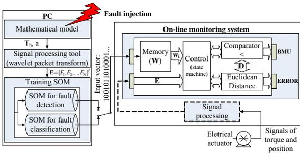
Figure 1. The proactive maintenance scheme.
