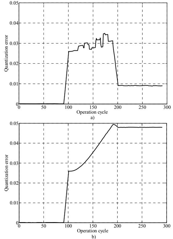
**Figure 5. Quantization errors for: a) degrading  $K_R$  and b) degrading  $K_M$ .**
