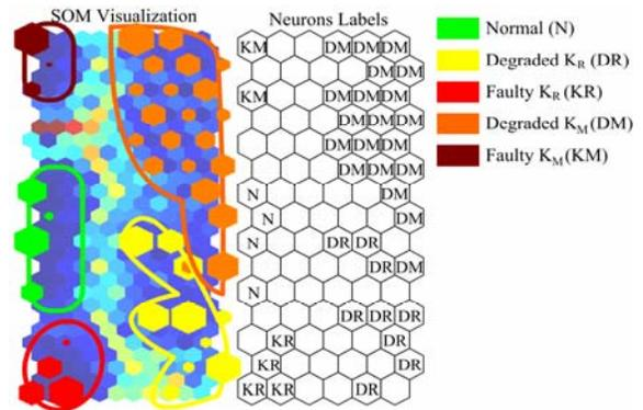
**Figure 6. Fault classification map considering faults in  $K_R$  and  $K_M$ .**
