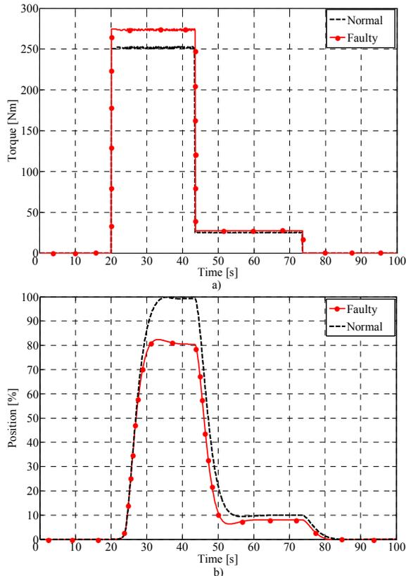
**Figure 4. Fault simulation: a) torque and b) opening position.**
