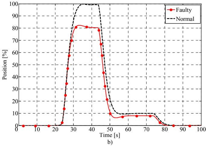
Figure 4. Fault simulation: a) torque and b) position.
