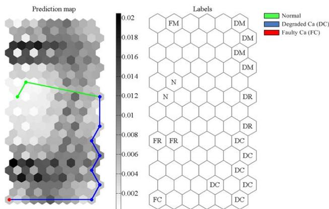
Figure 8. Fault prediction map considering faults in  $C_a$ .
