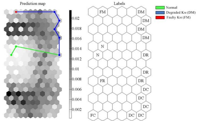
Figure 6. Fault prediction map considering faults in  $K_M$ .
