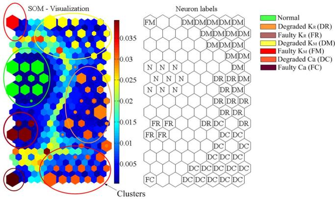
Figure 5. Fault classification map considering faults in  $K_R$ ,  $K_M$ , and  $C_a$ .
